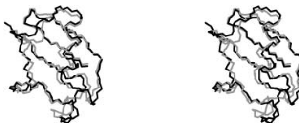
Figure 3. Stereoview of the global fold of human ubiquitin determined by using backbone residual dipolar coupling restraints and long-range amide–amide NOE restraints (black) compared with the crystal structure (grey). [36]
